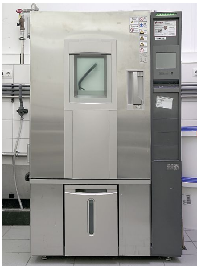
View of the test chamber for the climatic extremes test at -40°C/+80°C.
