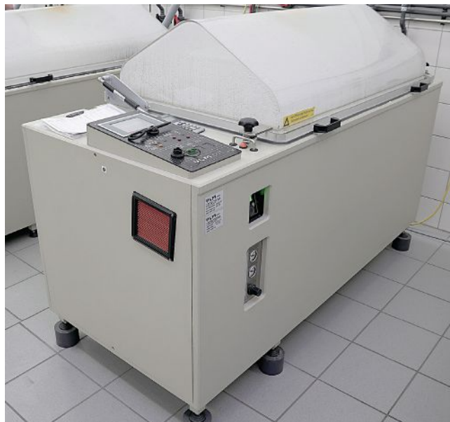
A test chamber for the conducting of neutral salt spray testing in accordance with ASTM B117/ISO 9227 NSS .
